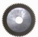
CUTTER NUMBER: 9010MC STYLE: MILLING CUTTER DIAMETER: 60MM THICKNESS: 7.3MM HOLE DIAMETER: 1/2" MAT: HIGH SPEED STEEL USE ON: JET 9010 with serial
